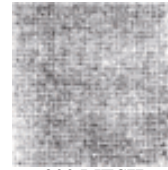
200 MESH Wire Dia. 0.0021 Opening 0.0029 34% Open Area
