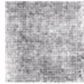
150 MESH Wire Dia. 0.0026 Opening 0.0041 37% Open Area
